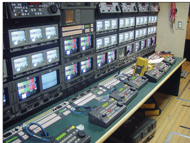
Figure 3.55 Tape compartment of the truck in Figure 3.54 as it approaches the testing phase. The controllers on the desk control digital VTRs above. Why all the monitors? So operators can see the video inot each VTR, along with what each is feeding back out, plus all the sources available that can be selected to be fed into the VTRs.
