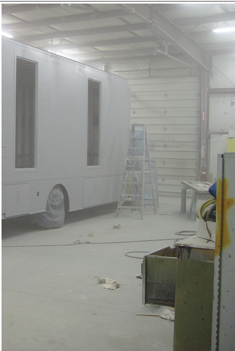
Figure 3.50 The truck or trailer is then primed and painted. Some manufacturers will paint the vehicle before the racks and inside finish is completed. Then any livery identifying the truck's owner, and often a major customer, is added.
