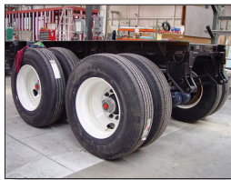
Figure 3.44 Every new remote truck must start somewhere — why not with a pair of axles? These two axles, along with leaf springs and shocks for suspension, will be fabricated into a trailer's running gear, also known as the "bogie."
