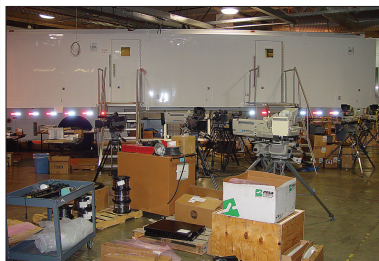
Figure 3.56 Equipment and cable are staged outside this trailer under construction awaiting installation. Also seen here are the trailer's complement of cameras, which will be tested as part of the overall system checkout. The closest camera facing away from the truck does not have a lens mounted on it yet.
