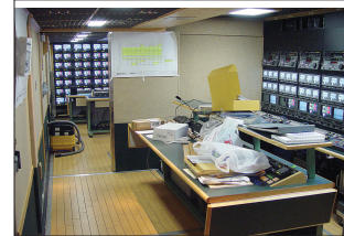
Figure 3.51 State of the art production trailer under construction. Foreground is tape compartment; in the distance is the production compartment's monitor wall.
